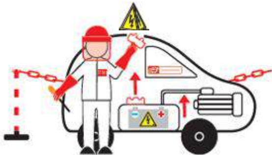
3) lock-out in "OFF" Position
