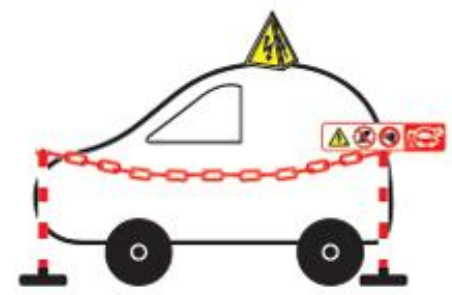
1) Identify the vehicle and the work area
