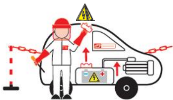
3) lock-out in "OFF" Position
